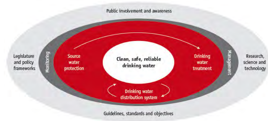
Figure 9 Multi-barrier approach to Drinking Water Safety (2)
